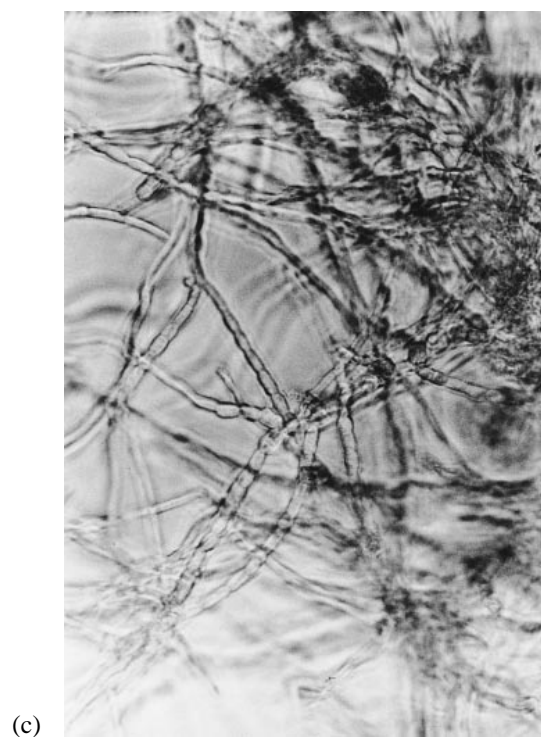
FIG. 2 Microscopic observations of the various activated sludge floc structures: (a) normal floc, (b) pinpoint floc, (c) bulking floc.
