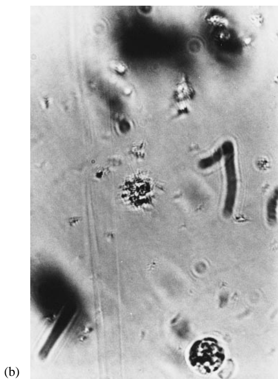
FIG. 2 Microscopic observations of the various activated sludge floc structures: (a) normal floc, (b) pinpoint floc, (c) bulking floc.
